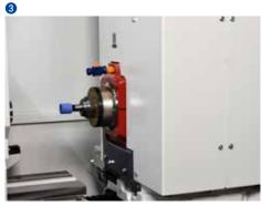
The S121 can be configured with a fixed spindle or a spindle turret with two spindles. The spindle turret swivels hydraulically through 180° to a stop. One spindle can be equipped with an external grinding wheel.
